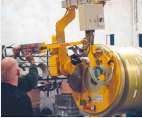
VacuCoil during removal process from a mandril
