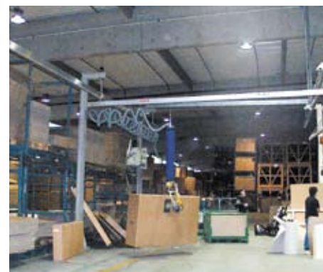
VPL with vertical suction foot for box handling
