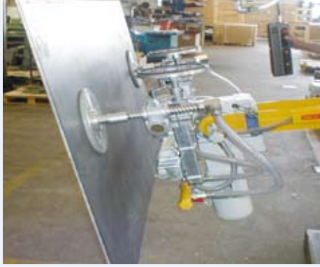
VacuBoy-180 with special attachment for the turning over of steel sheets
