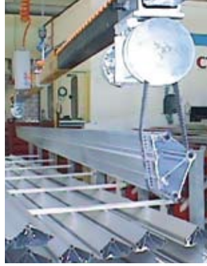
VacuBoy Tube with electric turn over for aluminium profiles
