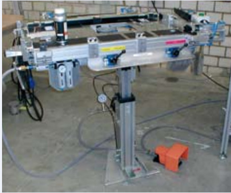
VacuStand with special attachment for pneumatic grippers
