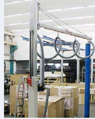
Slewing jib with telescopic post
