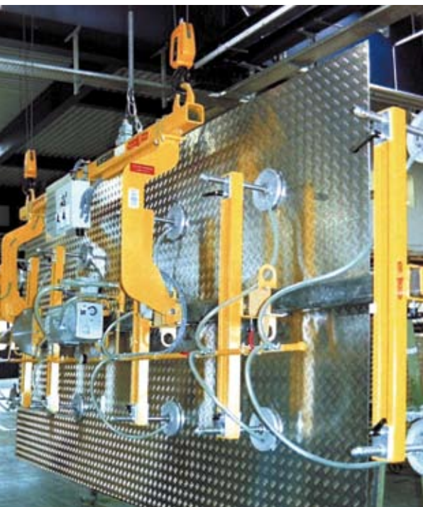
VacuGiant while handling chequer plates vertically
