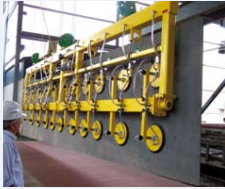
VacuGiant for the upright storage of plates in a shipyard
