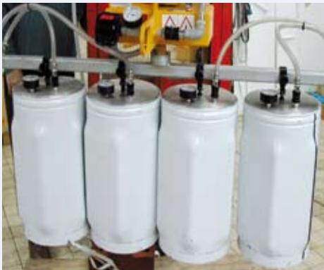
VacuBoy Mini with special assembly for handling of drums
