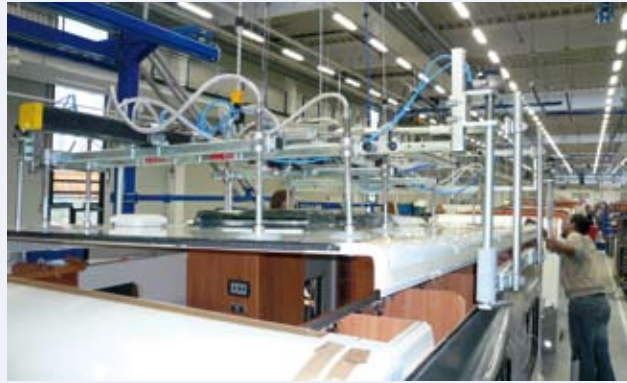
VacuBoy during the assembly of car roofs
