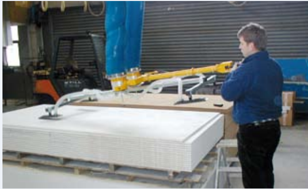
VPL with double tube while handling plaster plates
