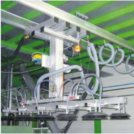
LiftFix for production of foam elements in an automated process
