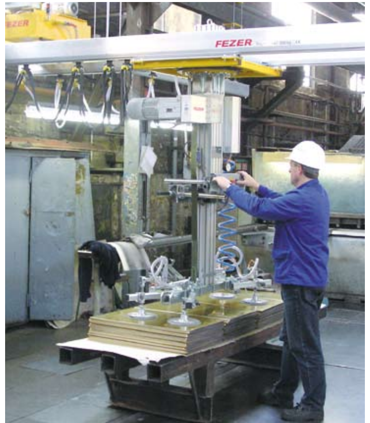
To-the-point feeding of a bending machine
