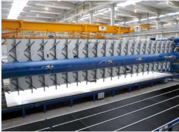
Turning station for side bodies of trucks with a length of 13500mm
