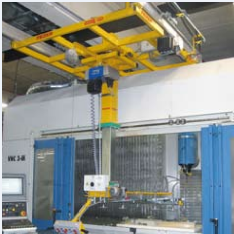
Exact feeding of a CNC machine
