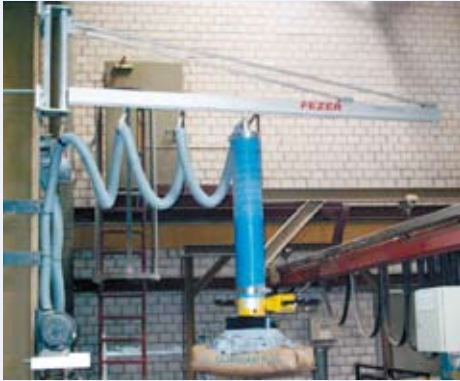
Wall slewing jib for sack handling
