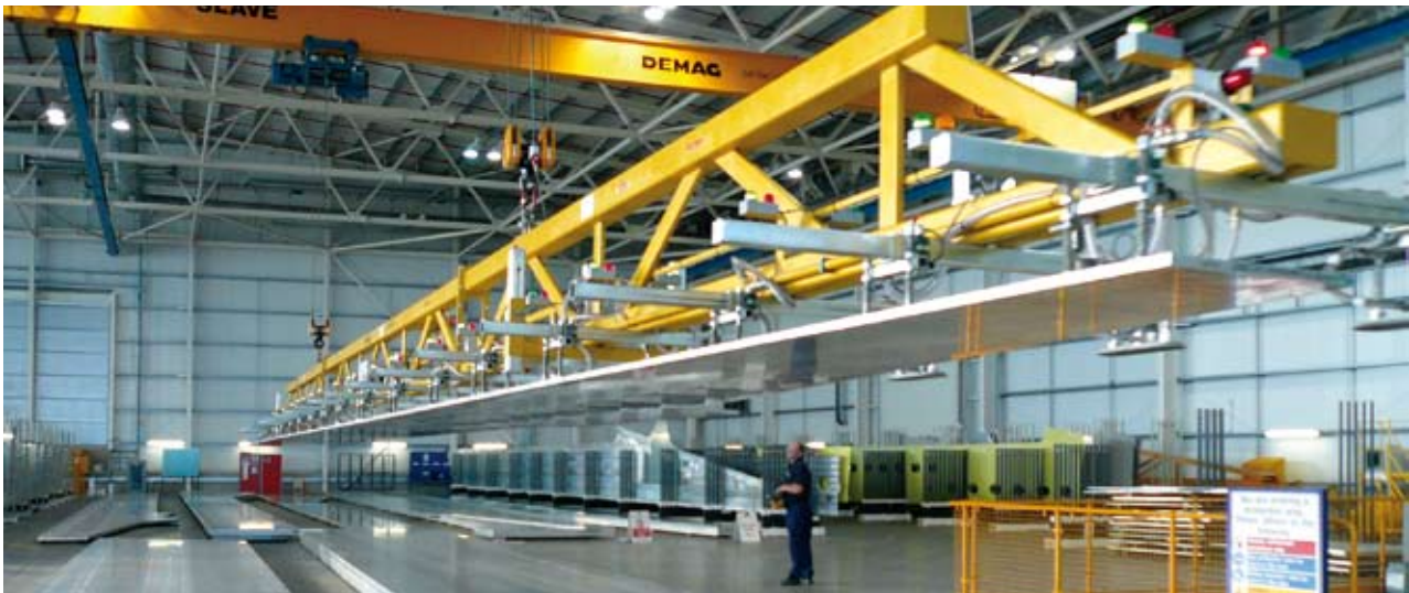
VacuGiant handling parts for airplane wings
