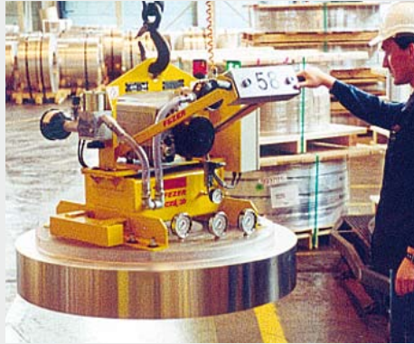
VacuCoil with transparent suction plate
