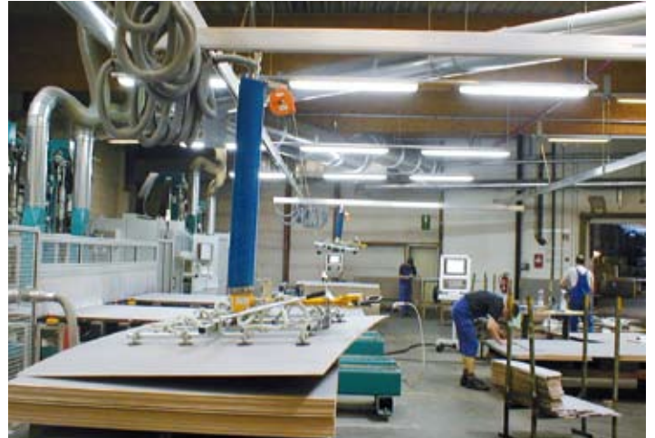
Single track system with several crane bridges for feeding CNC machines
