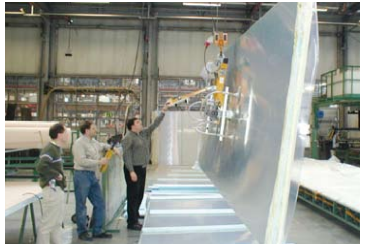
VacuBoy-90 handling wrapped sandwich elements
