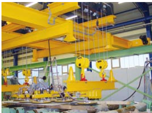
VacuGiant with four-point suspension and automatic crane
