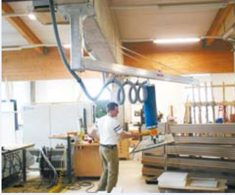
Slewing jib with ceiling suspension
