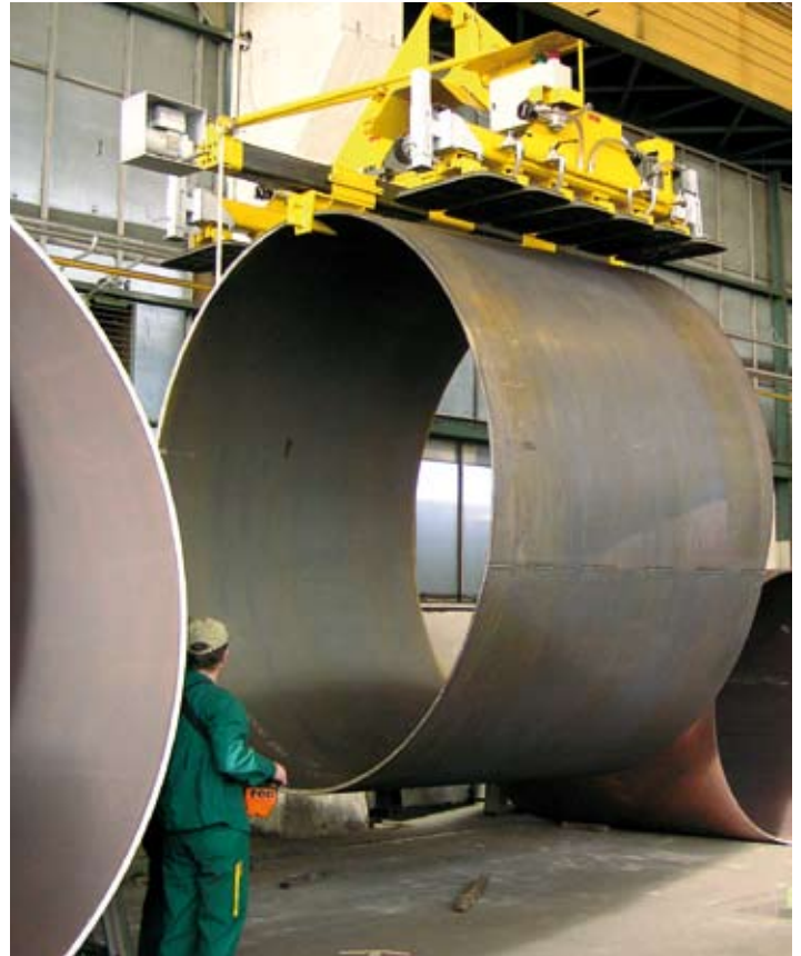
VacuGiant as "two-in-one" solution. Handling of steel plates and rolled tubes with a mechanical gripper solution
