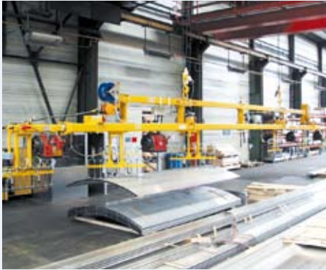
VacuGiant in special design with integrated rotation motors
