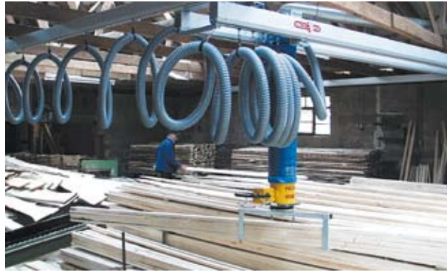
VPL with mechanical gripper for gluelam beams
