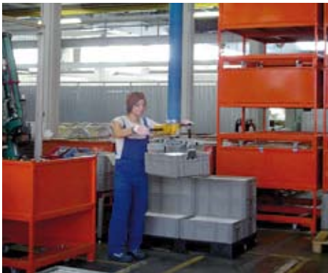
VPL with mechanical gripper for plastic boxes
