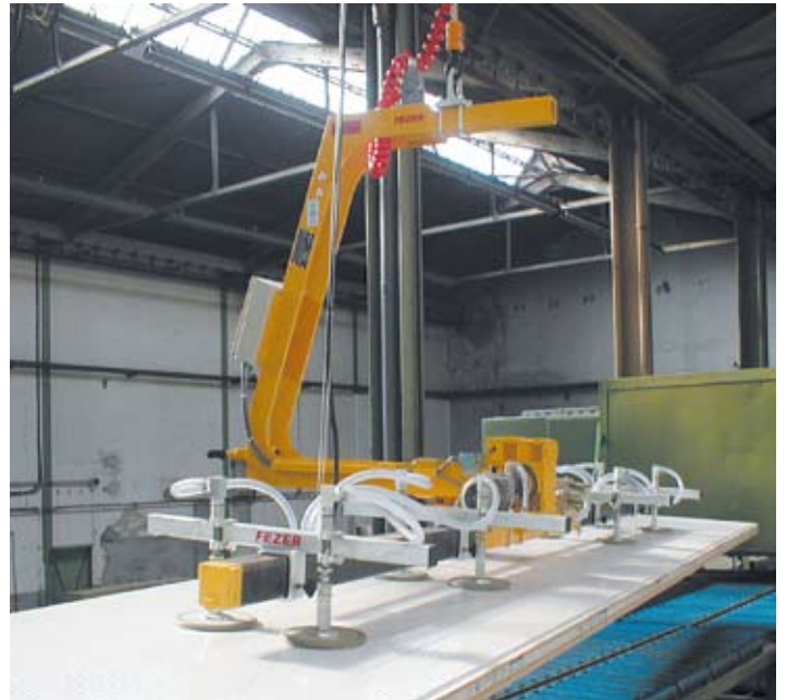
VacuBoy-180 for turning over sandwich plates
