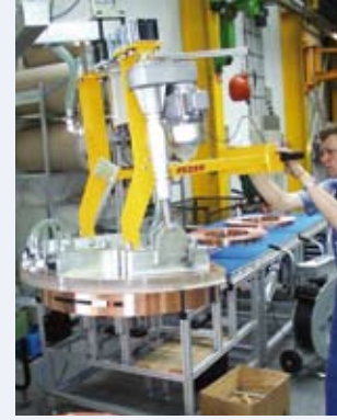
VacuCoil with transparent suction plate for the cable industry
