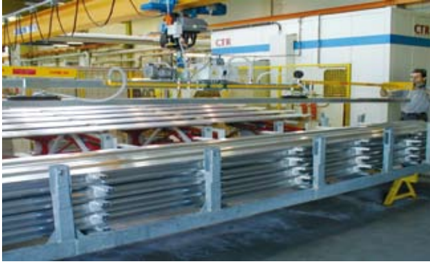
VacuBoy Tube handling aluminium profiles
