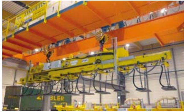
VacuGiant with electric extension for feeding plates
