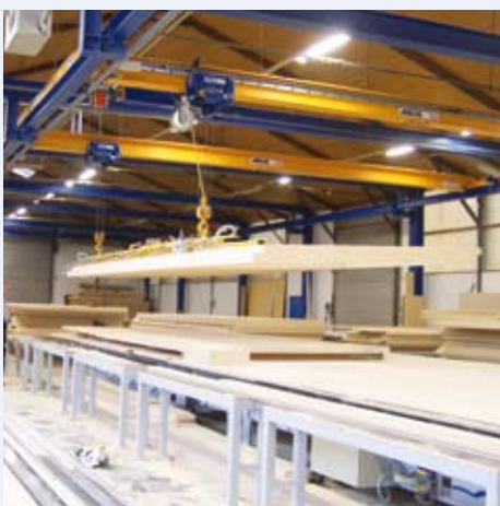
VacuPoro in special design for the manufacturing of prefab houses
