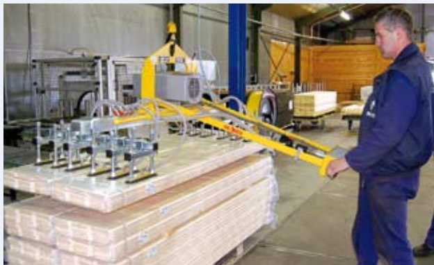
VacuBoy for horizontal handling of wrapped wooden planks
