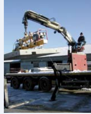
VacuGiant with generator for outdoor use
