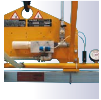
"Pneumatic Tool" for compressed air operation and pneumatic warning unit
