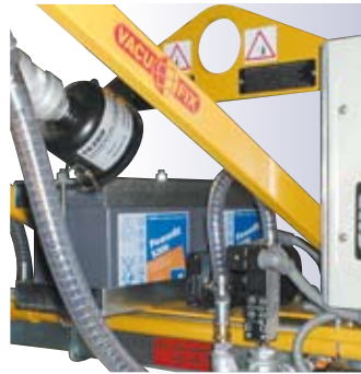
"Battery Pack" for power-independent operation by battery and charger
