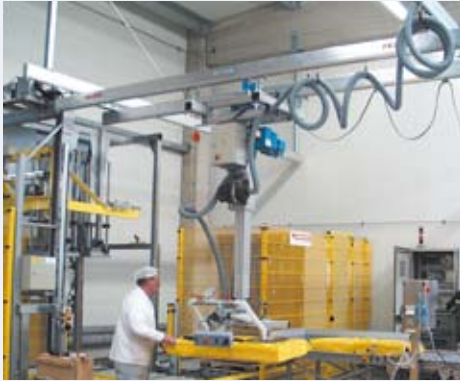
Area-wide suspension crane system for the food industry
