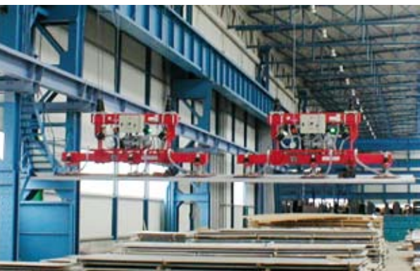
VacuGiant with synchronized tandem operation
