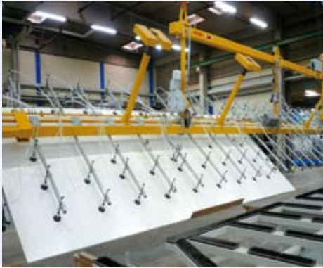
VacuGiant with swivel feature in both directions and counter weight for the precise 90° positioning of the plates
