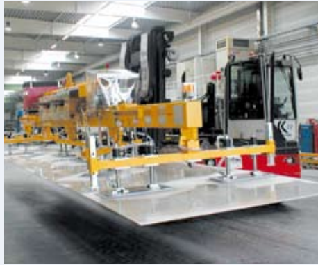
VacuGiant with generator for connection to a forklift truck
